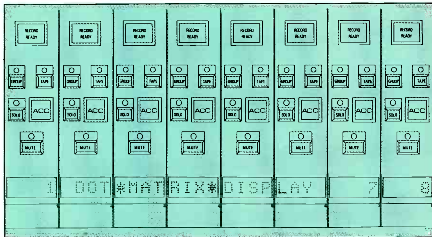
Figure 6. Individual access panels are provided for each monitor channel with stereo solo, mute, group, tape switching and record/ready selection.
