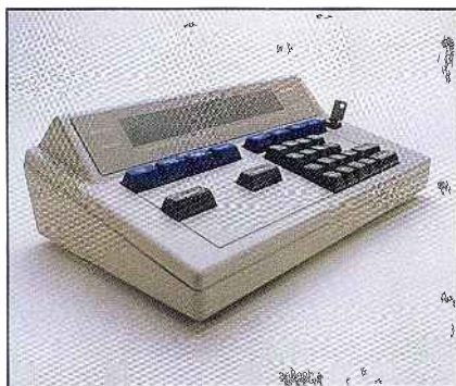
Various record and playback functions can be controlled from the remote-access station.
